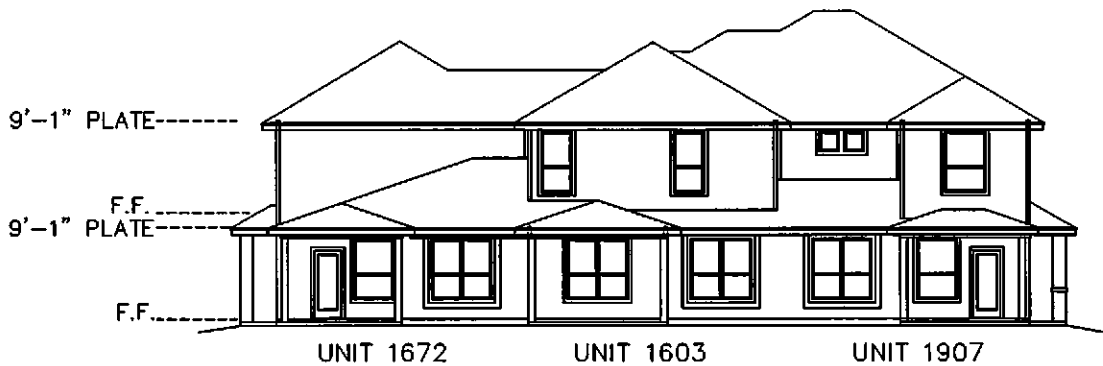
THREE-PLEX BUILDING 5182L REAR ELEVATION
